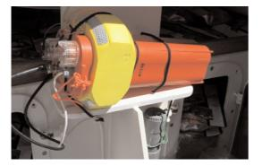
Argos is a **satellite** data collection and geo-location system. It can be used to locate transmitters (beacons) anywhere on the Earth's surface to within a position accuracy of +/- 150 meters (approx. 500 feet). Each beacon has a unique identification number and constantly emits its own signal.
